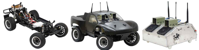
Fig. 2: AutoRally chassis and compute box [53].
