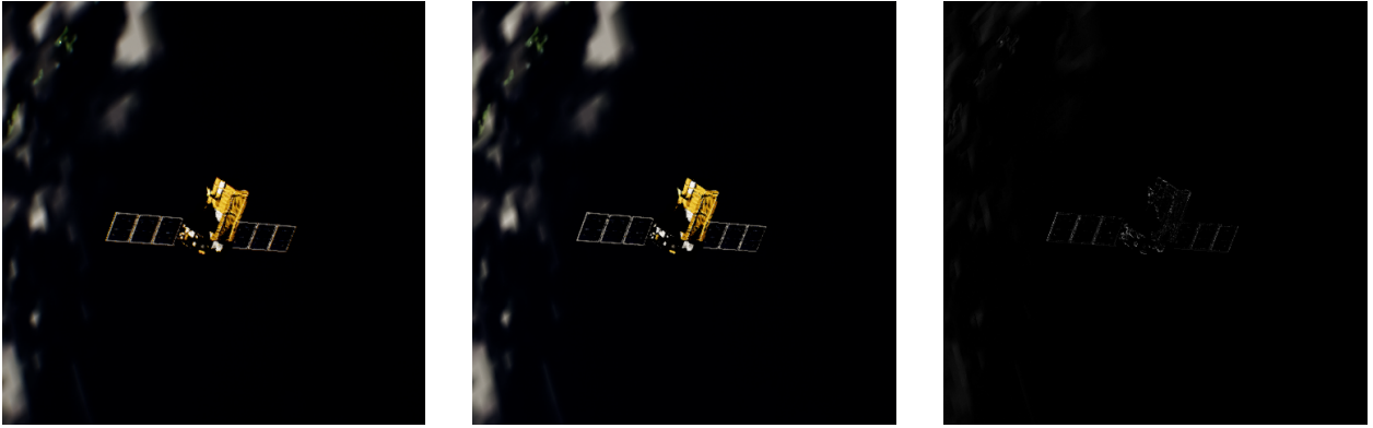
Fig. 8 Left: baseline image with the Earth partially in the field of view. Middle: same image with enhanced bloom effect. Right: pixel-wise difference between the baseline and the bloom-enhanced image.
