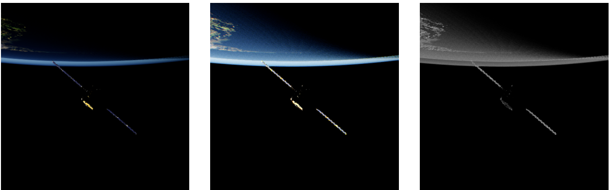
Fig. 10 Left: baseline image with the Earth partially in the field of view. Middle: same image with enhanced chromatic aberration intensity and film grain effects. Right: pixel-wise difference between the baseline and the enhanced image.
