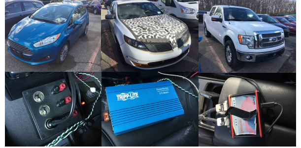
Fig. 3. Vehicles and apparatus used in the experiments. 1st row: Fiesta (left), MKS (medium), F150 (right); 2nd row: power source (left), power converter (medium), CAN case (right).
