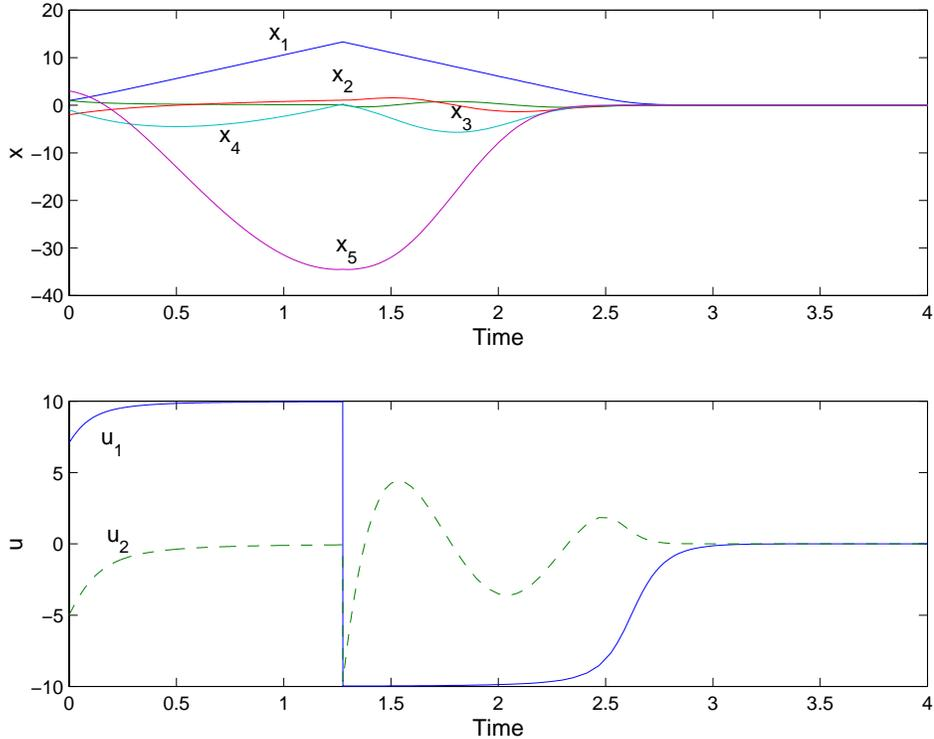
Fig. 2. History of states and control inputs with constraints.
