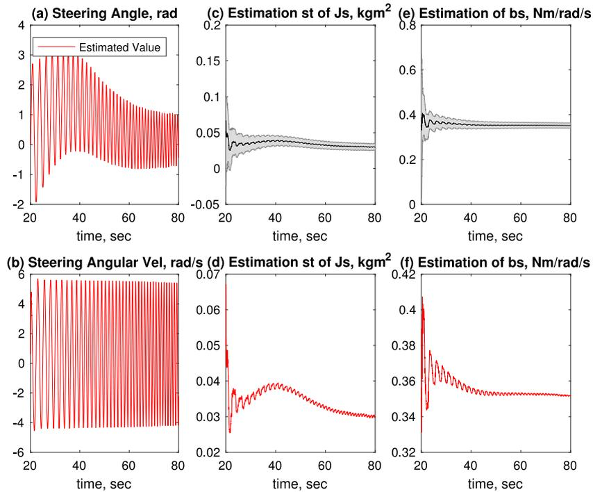
Fig. 5. System identification of the GTDS steering wheel using joint EKF.
