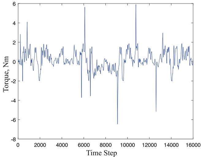
Fig. 13. Estimated driving torque to drive around the circuit clockwise (first half) and counter-clockwise (second half).
