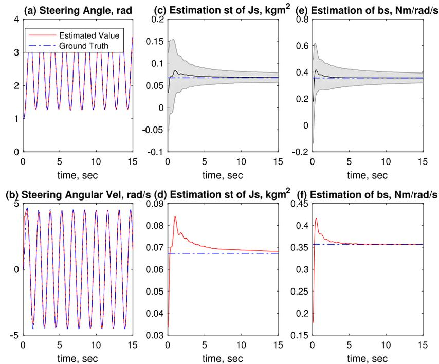
Fig. 3. System identification using joint UKF.
