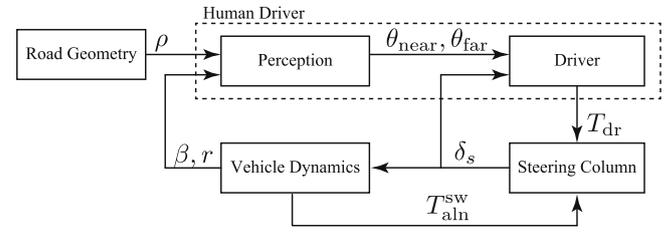
Fig. 1. The sensorimotor two-point visual control model framework.
