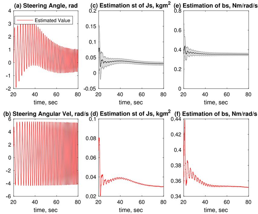
Fig. 6. System identification of the GTDS steering wheel using joint UKF.
