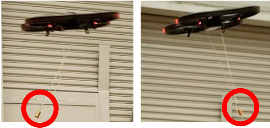
Fig. 6 Sling load generates significant model error and pendulous oscillation disturbance in flight.
