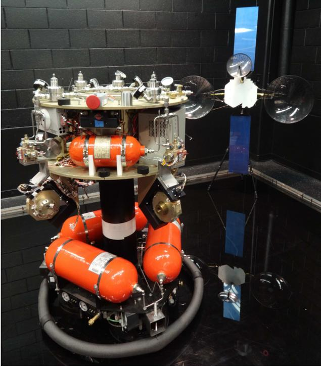
**Fig. 3** Five degree-of-freedom experimental platform of the ASTROS facility.
