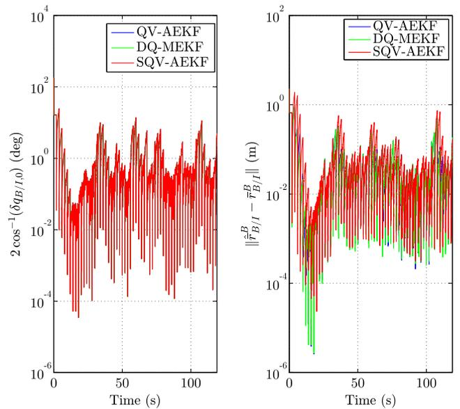
**Fig. 8 Case 1: pose estimation error (pose measurements at 0.5 Hz).**
