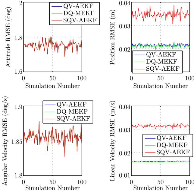
**Fig. 17** Rms state estimation error in simulations (pose measurements at 0.5 Hz).
