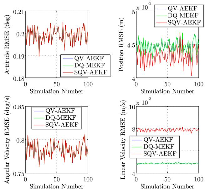
Fig. 16 Rms state estimation error in simulations (pose measurements at 10 Hz).
