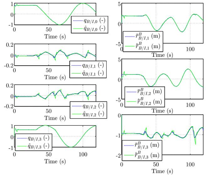
**Fig. 7 Case 1: estimated and true pose (pose measurements at 0.5 Hz).**
