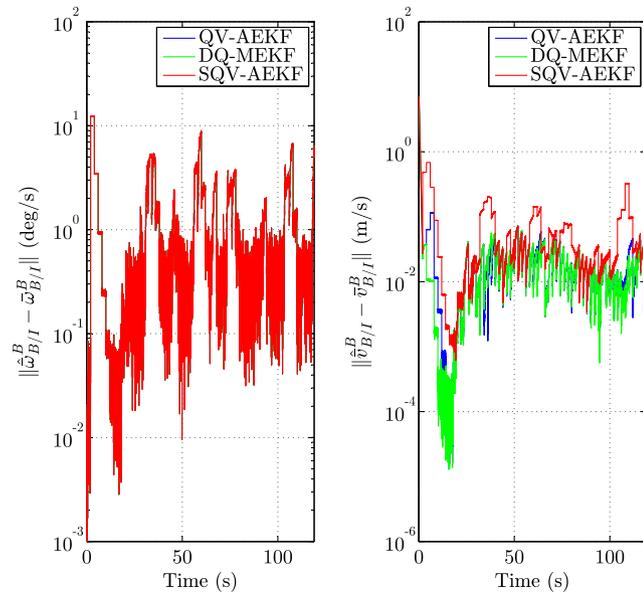
Fig. 9 Case 1: velocity estimation error (pose measurements at 0.5 Hz).
