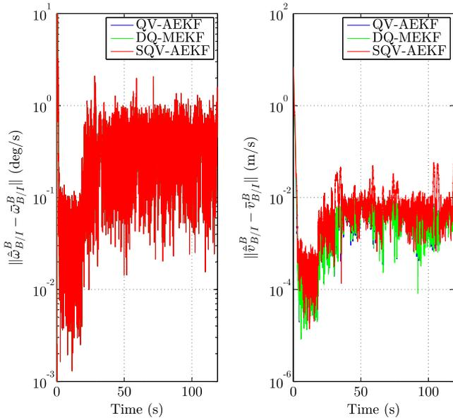
**Fig. 6 Case 1: velocity estimation error (pose measurements at 10 Hz).**
