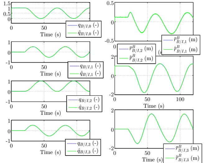
Fig. 15 Estimated and true pose (pose measurements at 10 Hz).
