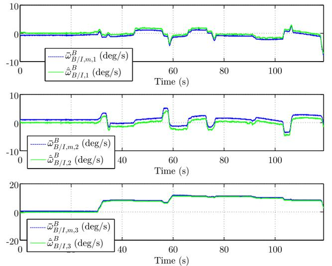
Fig. 11 Case 2: estimated and measured angular velocity.
