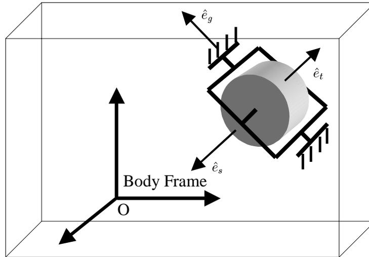
Figure 1: Spacecraft Body with a Single VSCMG
