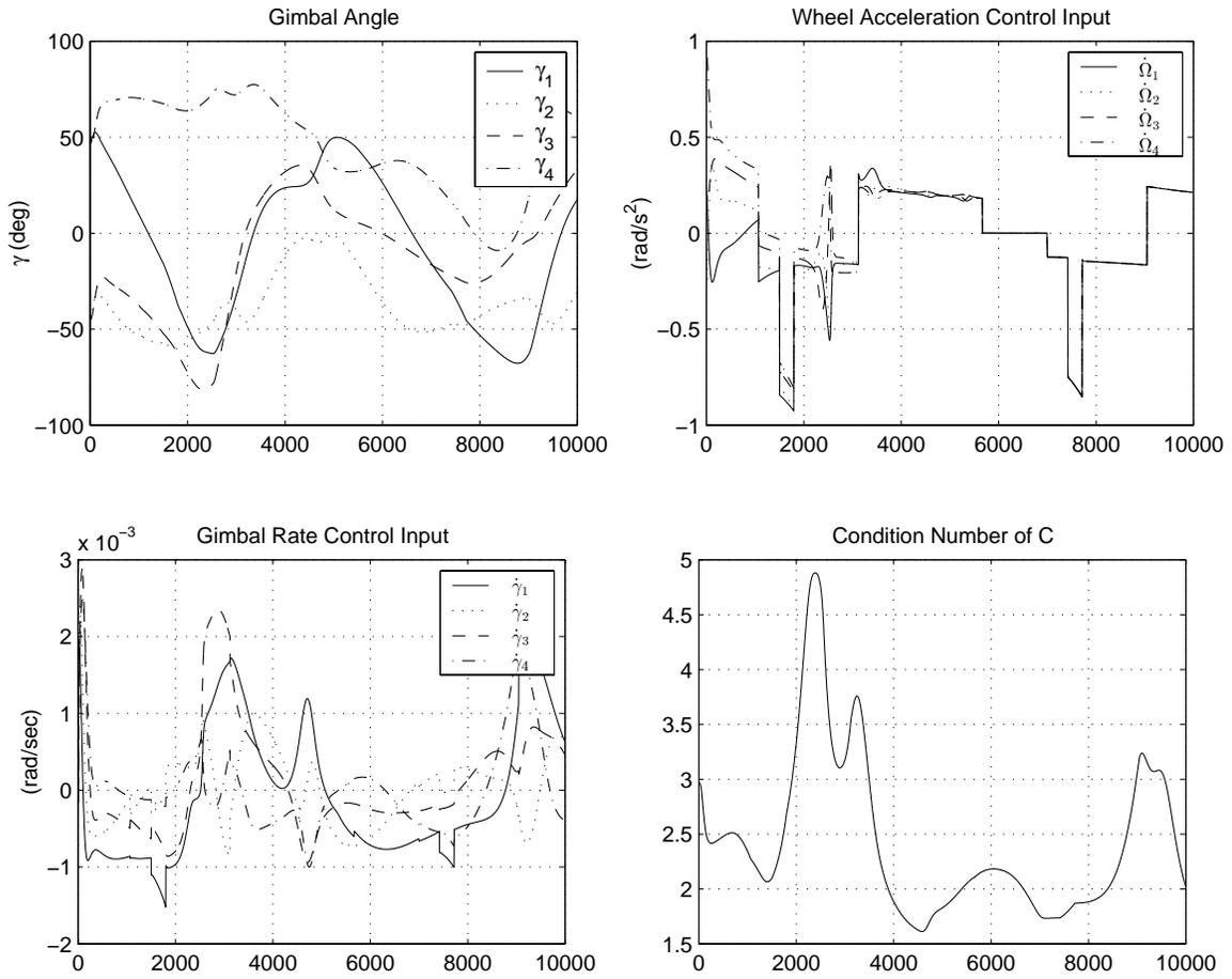
Figure 5: Gimbal Angles, Control Inputs and Condition Number of Matrix  $C$  (Method 1)
