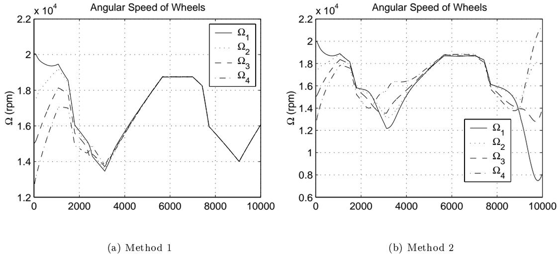
Figure 4: Angular Wheel Speeds with Speed Equalization
