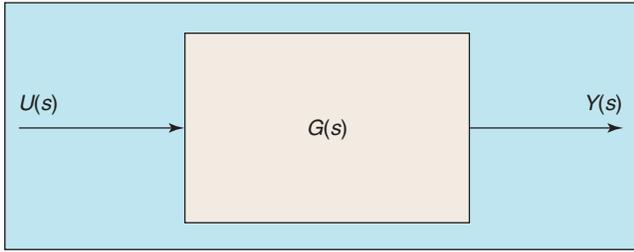
**Figure 2.** A block diagram for a single-input, single-output system. The transfer function  $G(s)$  is defined as the ratio of the Laplace transform of the output signal  $Y(s)$  to the Laplace transform of the input signal  $U(s)$ . For linear time-invariant systems the transfer function  $G(s)$  is independent of the choice of input  $U(s)$ .
