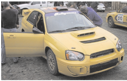
Fig. 1. The 340 BHP, 510 Nm, All-Wheel-Drive CPD Racing Subaru Impreza.
