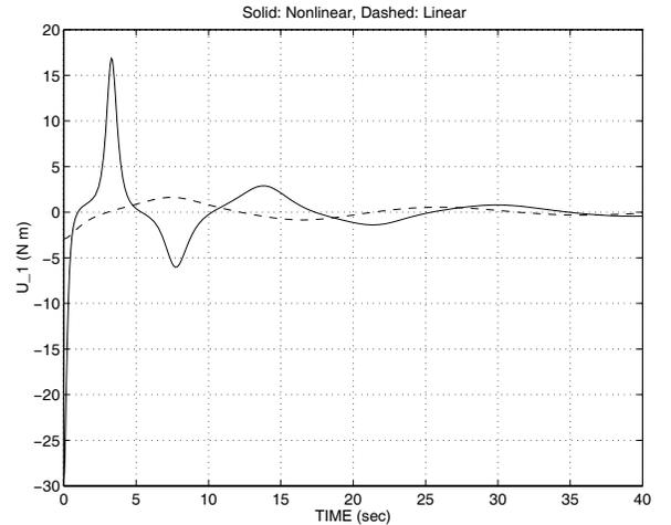
Fig. 2 Controller comparison; Control history for Rodrigues parameters.
