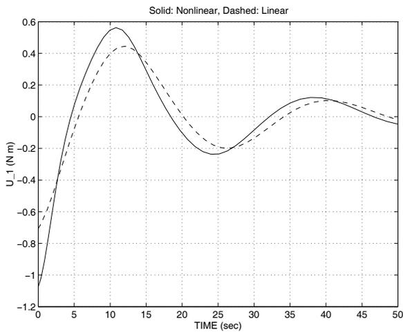
Fig. 4 Controller comparison; Control history for Modified Rodrigues parameters.
