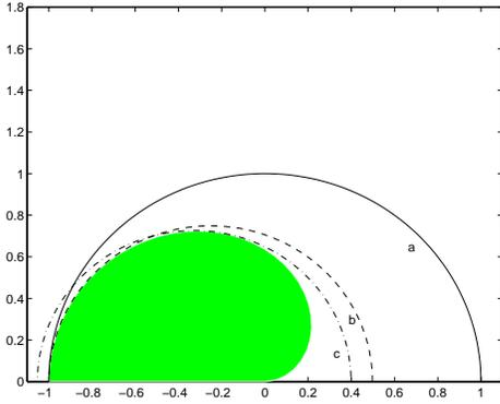
**Figure 3:** Delay element value set  $\Phi_1$  (shaded) and covering disks. (a) Unit disk  $\mathbf{B}$ . (b)  $\mathbf{D}(-0.251; 0.749)$ , the disk with minimum radius among all contained within  $\mathbf{B}$ . (c)  $\mathbf{D}(-0.327; 0.726)$ , the minimum radius covering disk.
