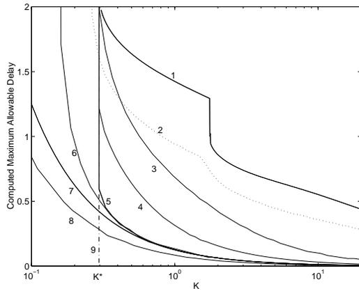
**Figure 6:** Maximum delay margin vs.  $K$ . (1) Actual value from Nyquist Criterion. (2) Theorem 3 with filter (14) and covering disk  $\mathbf{D}(-0.496; 0.504)$ . (3) Theorem 3 with filter (9) and covering disk  $\mathbf{D}(-0.51; 0.637)$ . (4) Theorem 1 with covering disk  $\mathbf{D}(-0.327; 0.726)$ . (5) Result of [13]. (6) Theorem 2 with filter (9). (7) Result of [9]. (8) Result of [11]. (9) Delay-independent result [18].
