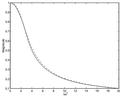
**Figure 4:** Frequency response of filter (9)  $|f(j\omega)|$  (dashed) and  $g(\omega)$  (solid).
