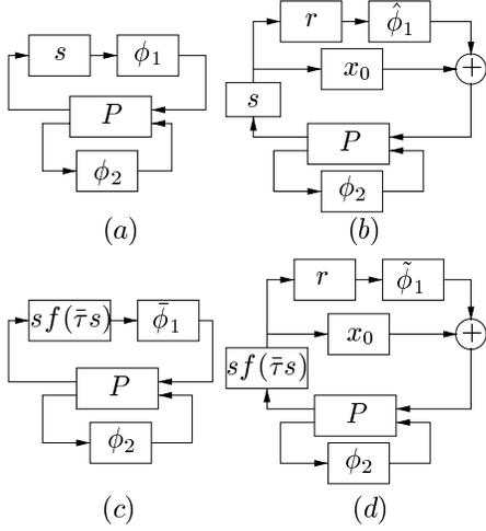
**Figure 2:** Loop transformations. (a) System (4). (b) With shifted disk. (c) With filter. (d) With both filter and shifted disk.
