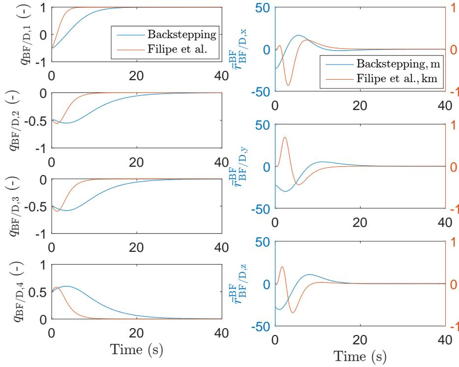
Figure 3. Relative pose between follower and desired reference frames.
