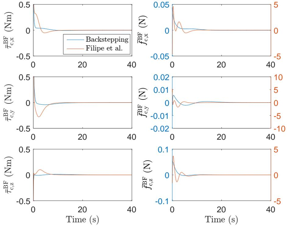
Figure 5. Control forces and torques applied by the follower spacecraft.
