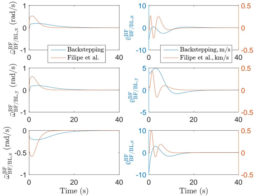
Figure 4. Relative linear and angular velocities between follower and leader spacecraft body frames.
