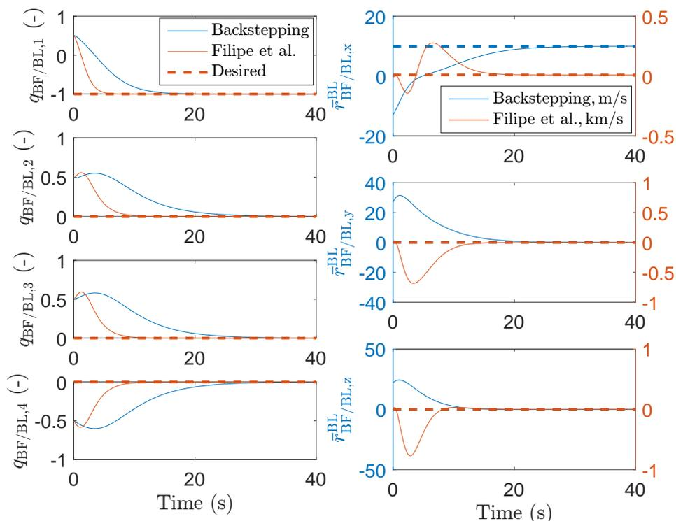
Figure 2. Relative pose between follower and leader spacecraft body frames. (Dashed lines show desired frame pose:  $q_{D/BL}$ )
