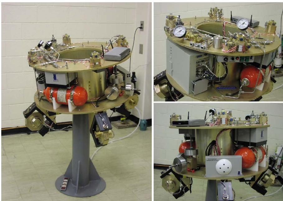
Figure 1. The Georgia Tech three-axial spacecraft simulator.
